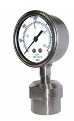
Diaphragm Seals are designed for use in applications where chemical compatibility, trash or sludge in process or sanitary requirements prevent the use of a standard pressure gauge or gauge only installation.
